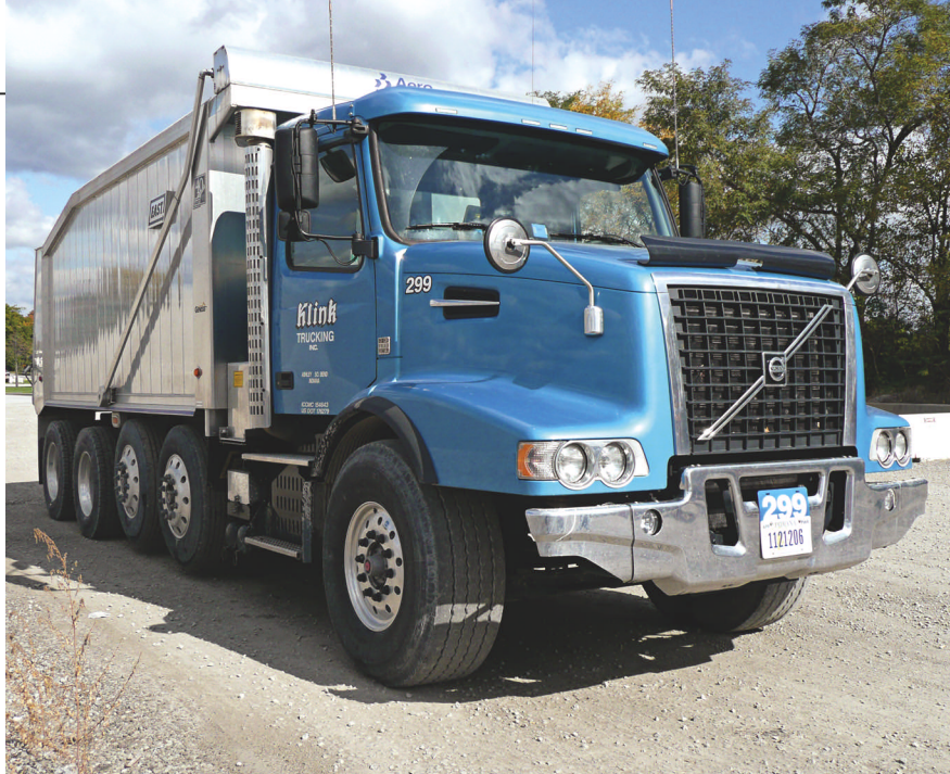
As equipped with its two pusher axles, Number 299 can legally gross up to 73,280 pounds in Indiana. An East smooth-sided aluminum dump body helps maximize payload.
