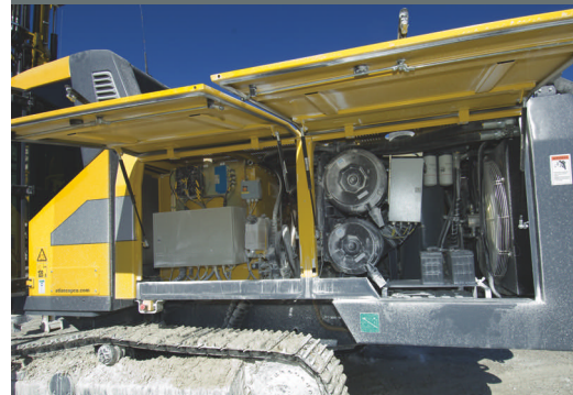
Backup batteries were added to the latest version of the F9C and are accessible from the ground on the left side, along with air filters.
