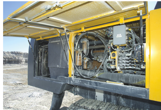
Collecting oil, fuel and hydraulic filters behind the ROC F9C's right-side access panel eliminates the need to climb up on a track for regular maintenance.
