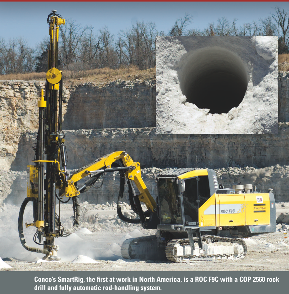
Conco consistently plans 4-inch, vertical blast holes. Double drill-steel support in Atlas Copco's drifter guides the bit accurately for consistent collaring and straight holes.
