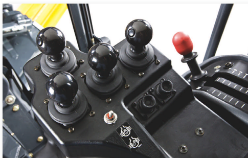
Levers (right to left) on the right-armrest console control blade lift (button: blade control on/off), wheel lean, draft-frame side shift, and the front lever controls articulation (button: return to straight).
