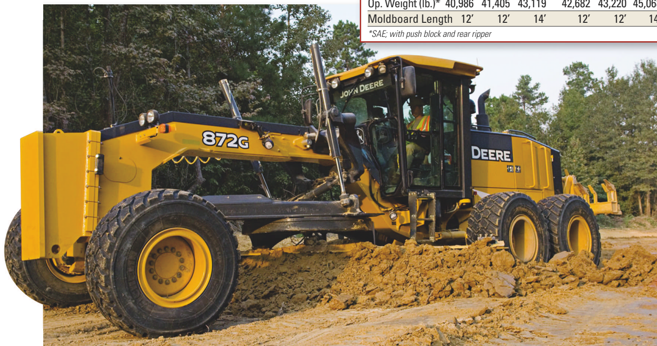
The G Series offers a lot of choices: electronic or hydraulic controls; wheel or wheel-and-lever steering; Topcon or Trimble grade control; tandem or all-wheel drive; front, mid-mount or rear ripper/scarifier.
