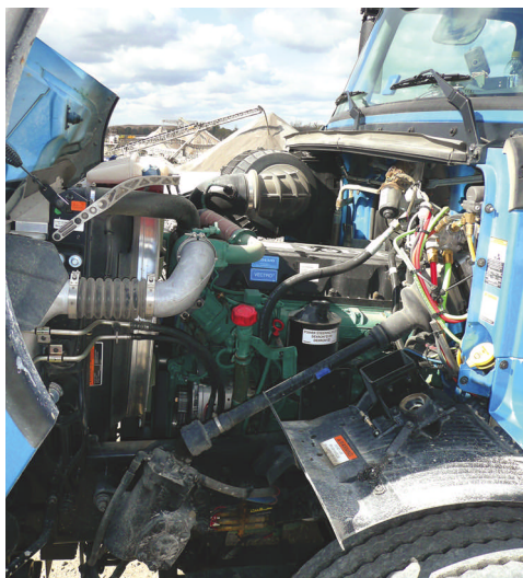
VHDs don't offer a choice of engines; the 12.8-liter Volvo D13 is the only one available.
