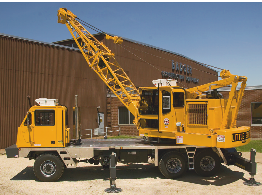
Little Giant Corp. offers the 30-ton-capacity Little Giant 6430, a carrier-mounted, lattice-boom crane that it claims can be optioned to an “all-terrain” model.
