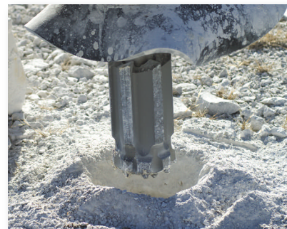
Conco consistently plans 4-inch, vertical blast holes. Double drill-steel support in Atlas Copco's drifter guides the bit accurately for consistent collaring and straight holes.
